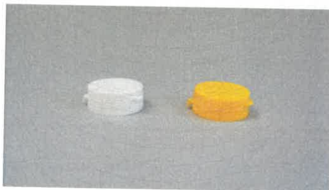
Fig. 1 – delivered sample – Plastic caps made of PE RIBLENE MR 10R FE S312 (white, yellow)
